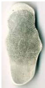
Figure 5 White silicone lift from textured surface (computer)
